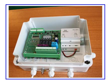
CAM99 unit installed in electric board with its voltage supply unit.
